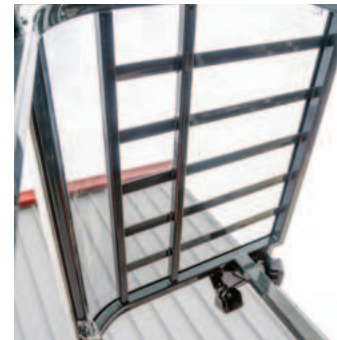
All-weather glass overhead guard cover
